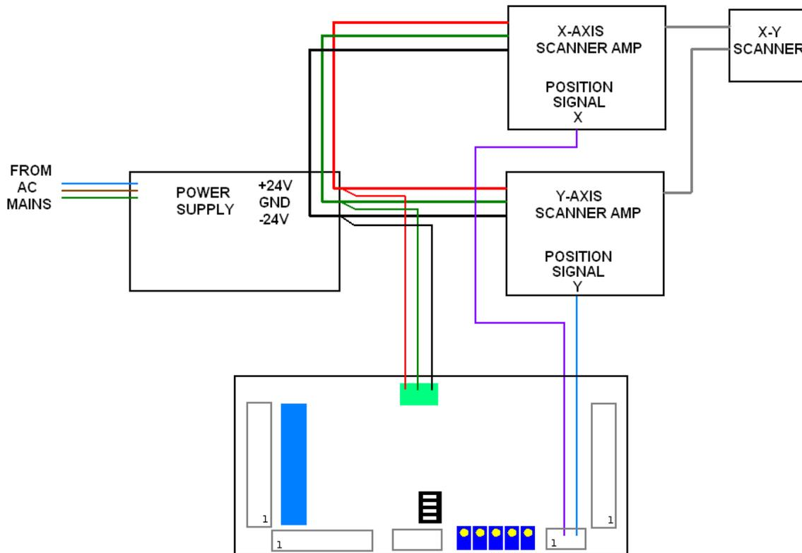
PASS monitors the power supplies that feed the scanner amplifiers. This voltage can be between +/-20 volts and +/- 30 volts. The manner in which you connect PASS to the power supply and to the scanner amplifiers depends heavily upon whether you are using two separate single-axis scanner amplifiers, or one dual-axis scanner amplifier.
